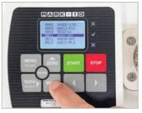
▲ Save and recall multiple profiles, for quick and accurate switchover to different test methods.
