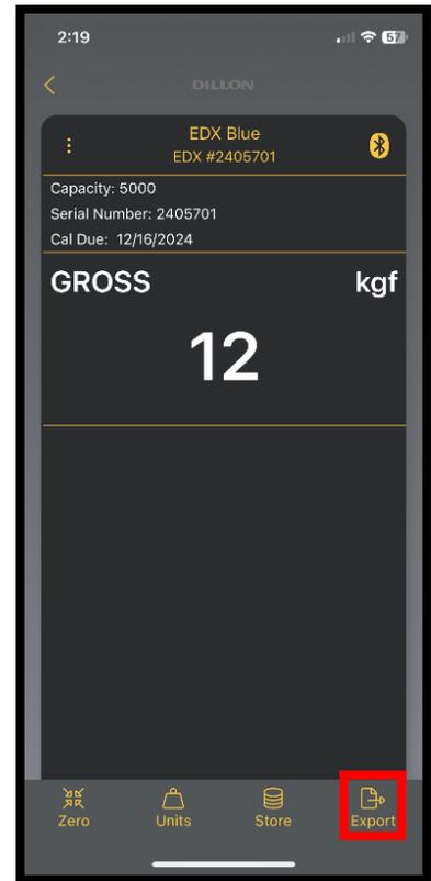
This will take you to a screen with the stored data page with the option to export as a PDF or Excel file. The logs will contain stored force readings with units and time stamps, as well as noting the unit's serial number, capacity, and calibration due date. Users can export the information in any format supported by the mobile device (email, airdrop, iMessage, text message, etc.)
