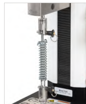
Tension spring testing
