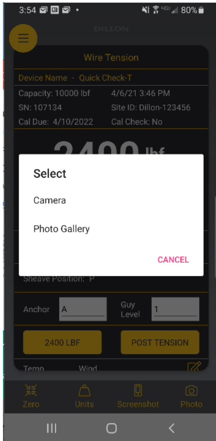
16. After the Guy Wire has been tensioned to target, the **Post Tension** button can be pressed to store the final tension to the Anchor and Guy Level selected. The value of the Post Tension reading will show where the Post Tension button used to be.
