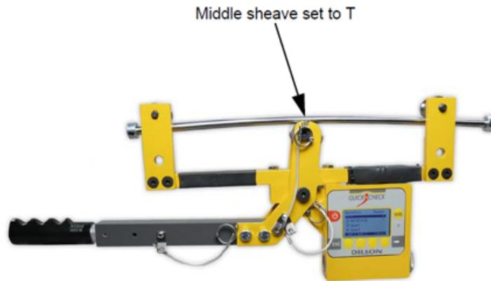
6. Clamp the Quick Check-T onto the calibration rod. Be sure the rod is riding in the center groove of all three sheaves, as shown above.
