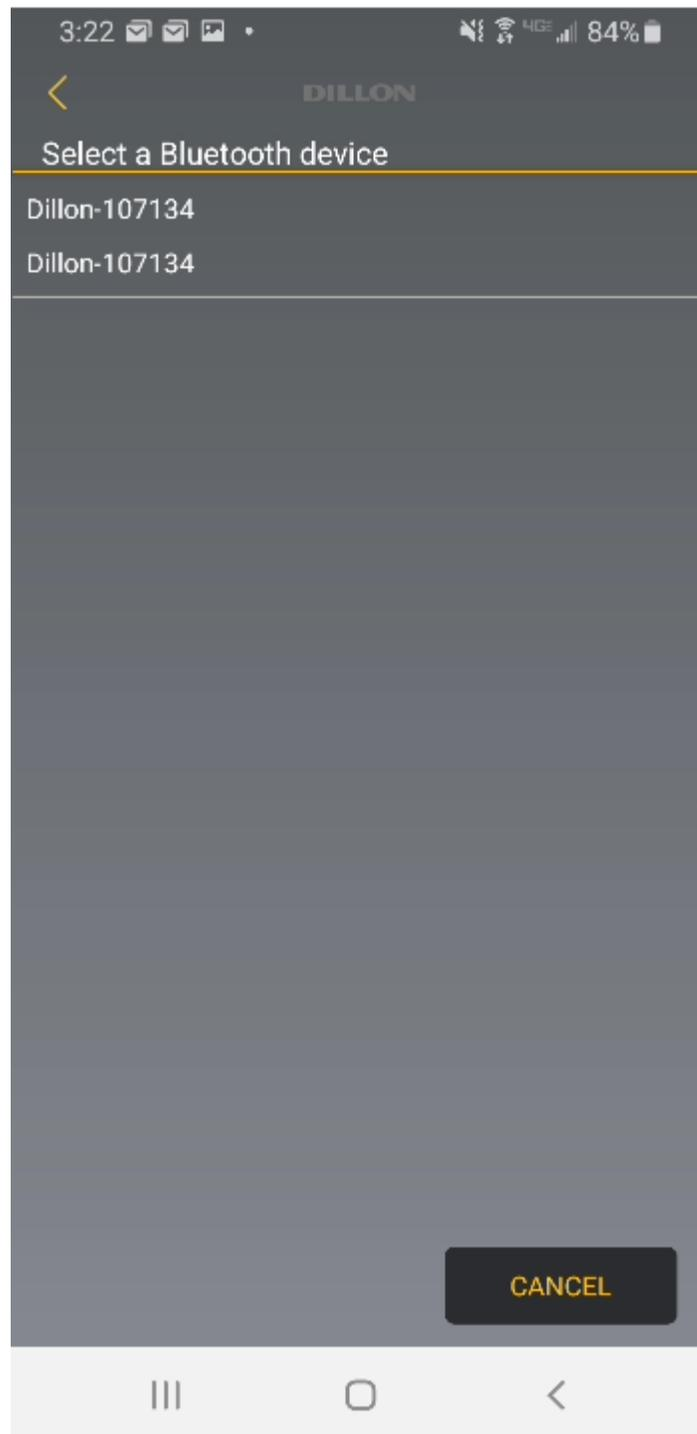
6. Select the Dillon-Serial Number of the device you want to connect to and **Name the Device**, then press **OK**.
