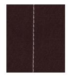
Seam with correctly adjusted thread tension
