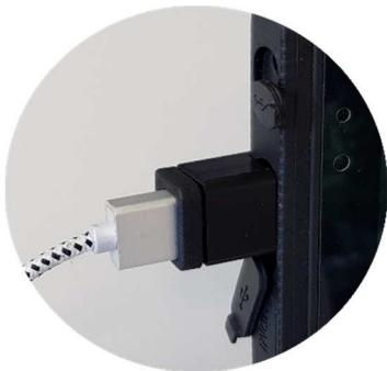
Connect the USB sensor connector to the USB-Port (3) of the tablet.
