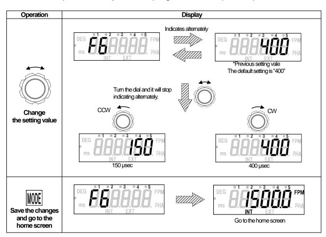
In function mode 6, the pulse width of the synchronous output signal can be set to 400 µsec or 150 µsec.
