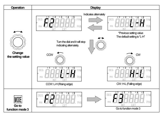
In function mode 2, in which the edge of the external pulse triggers emission, the rising edge or falling edge, can be set (for EXT).
