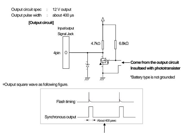
Pulse width can be changed in function mode 6 ( $\Rightarrow$ 150 µsec)
