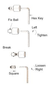
The break-away safety adapter is inserted into the square opening of the torque multiplier.
