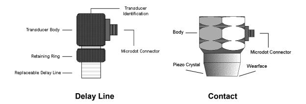
The Transducer is the "business end" of the *PZX-7 DL*. It transmits and receives ultrasonic sound waves that the *PZX-7 DL* uses to calculate the thickness of the material being measured. The transducer connects to the *PZX-7 DL* using a single shielded coaxial cable with microdot connectors.
