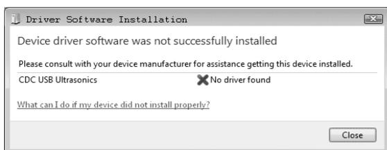
The driver file that needs to be installed can be found by installing our DakView PC software, and located in the USB directory. The file name is CDC\_Ultrasonics.inf, and can be downloaded and saved anywhere on your local PC.
