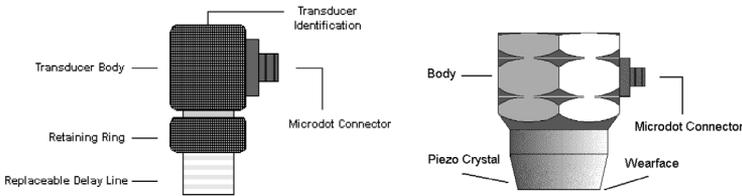
The transducer is the “business end” of the TI-007X. It transmits and receives ultrasonic sound waves that the TI-007X uses to calculate the thickness of the material being measured. The transducer connects to the TI-007X via a single shielded coaxial cable with microdot connectors.
