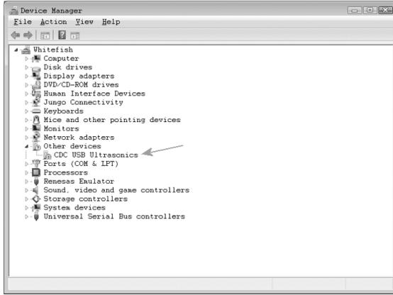
Select “browse my computer” and navigate to the directory where the driver was saved on your PC and install the driver. When the installation is completed, the following window will be displayed:
