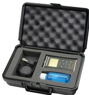
**Complete Kiti includes:** TI-25MX gauge, probe, 4 oz. bottle of coupling fluid, 2 AA batteries, NIST-traceable calibration certificate and operating instruction manual—all in a foam-fitted carrying case.
