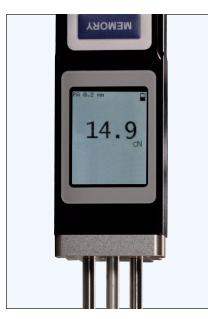
Depending on the measuring position, the color LCD display automatically rotates in 90° increments for optimal viewing.
