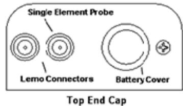
**NOTE:** There is no polarity associated with connecting the transducer to the TI-25SX, it can be plugged into the gauge in either direction.
