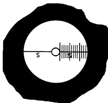
Fig. 2: Measurement of a film section consisting of a single layer using microscope
