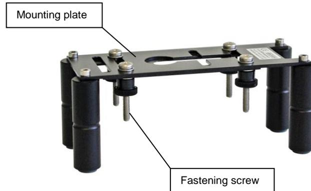
Slots are milled into the mounting plate of the specimen platform. These in conjunction with two rails with holes provide sufficient degrees of freedom for fixing specimens various geometrical shapes. When clamping the specimen take care that the mounting plate is not bent.
