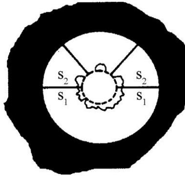
**Fig. 3: View through microscope onto drilled cut out with crumbled edges**
