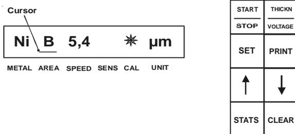
The instrument can be adjusted by pressing SET (6) and ARROW-(5) keys. For setting into selection mode, press SET-key. The position of the red cursor on the alpha-numerical display indicates the parameter which is to be set (e.g. de-plating speed or metal selection). Use the ARROW-keys for setting the required parameter. The parameters set by the ARROW-keys will be directly accepted. For quick setting, keep SET- or ARROW-key pressed down continuously (Quick function).
