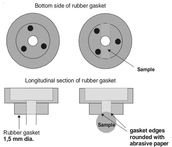
The rubber gasket *B* should not be adapted to the diameter of sample as this would change its defined measuring area.
