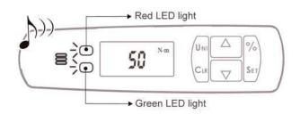
When applied torque exceeds the wrench full-scale capacity, the GREEN & RED lights are on and the buzzer beeps continuously. Display shows " ----"
