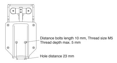
Optionally, the tension meter can be delivered with distance bolts for stationary use. The dimensions are given in the figure above. The distance bolts can be removed.
