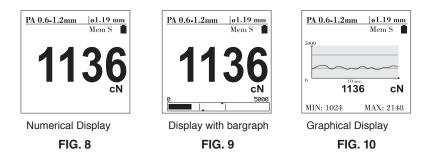
6. Press the ▲ and ▼ button simultaneously to change the different display modes during the working mode.
