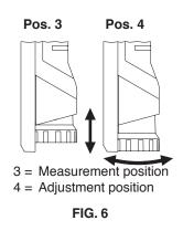
of the material thickness compensator back to the measurement position (Figure 6). If you set a diameter that has not been calibrated for the selected material characteristic, the set diameter is displayed with a black background color, e.g.,  $\emptyset 0.26mm$  the tension meter can be used anyhow, but please note, that depending on the material to be measured, slight deviations in the measured values might occur.
