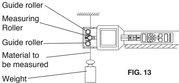
**NOTE:** While performing the calibration, the tension meter must be fixed in such a way that the material to be measured runs smoothly between the guide rollers and the measuring roller. The display gives detailed information on the calibration.
