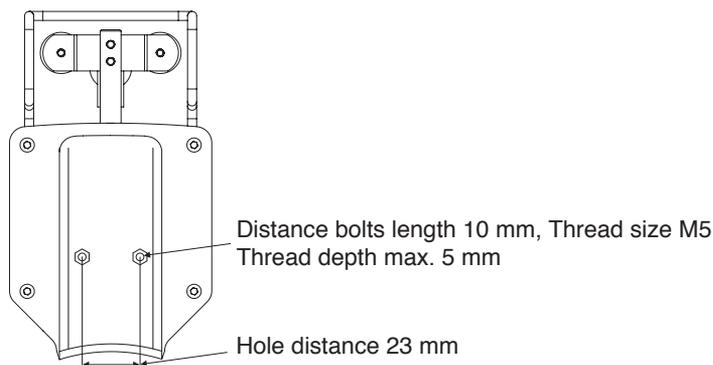
Optionally, the tension meter can be delivered with distance bolts for stationary use. The dimensions are given in the figure above. The distance bolts can be removed.
