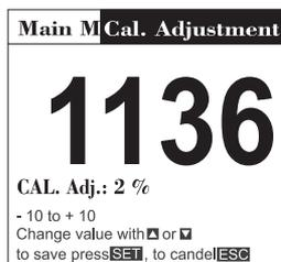
**NOTE:** Please note that this is a general value. So determine it separately for each material characteristic and note it down for later reference. It is not possible to save it per material characteristic.
