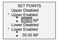
One, two, or none of the set points may be enabled. To toggle between the tension and compression directions, press the **DIRECTION** key.
