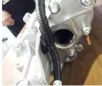
Limited access EPS Rack
