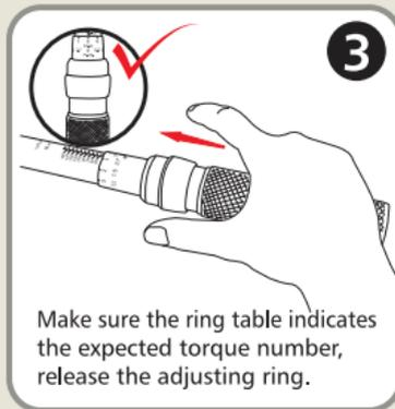
Make sure the ring table indicates the expected torque number, release the adjusting ring.
