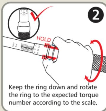
Keep the ring down and rotate the ring to the expected torque number according to the scale.
