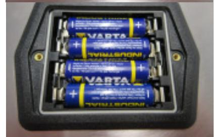
If the battery symbol appears in the measuring window resp. if a critical charge of battery is shown in the status, the batteries have to be changed IMMEDIATELY.
