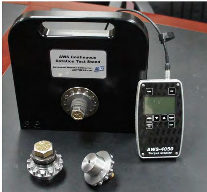
Frame with mounted transducer, rundown fixtures, AWS 4050 and transducer cable.
