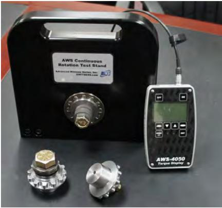
The AWS 41 Series Impact test stands are designed to test Impact and Pulse tools without experiencing damage to the torque transducer. We accomplish this by using a unique, AWS designed, S-spline transducer, which accurately measures and records the torque delivered by the tool being tested. The transducer is mounted into a frame that needs to be secured to a bench or sturdy work table.
