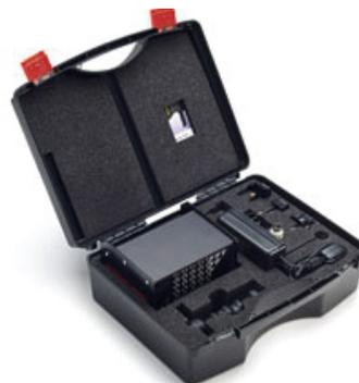
The QBS-LED is supplied as a complete kit including the strobe, removable handle, universal AC adapter with USA, EURO and UK plugs, DIN connector when using external trigger signal from sensor, traceable calibration certificate in a foam-fitted plastic carrying case.
