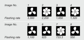
The orientation marking confirms that the images at 3,300, 1,650 and 825 rpm are harmonic multiple images. Three identification marks appear in each of these images.
