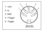
Fig. 3 - Assignment of the connection socket.
