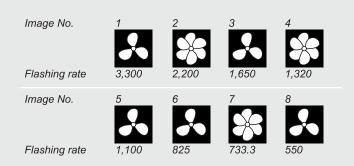
What is the actual rotational speed of the fan? Images 1, 3, 5, 6 and 8 correspond to the original one, which means the rotational speed could be 3300, 1650, 1100, 825 or 550 rpm.
