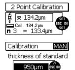
If the shown set point (Cal) as displayed is not identical with the thickness of your precision standard, use arrow up and down keys to adjust accordingly.
