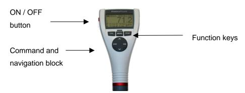
Press **ON/OFF** button to switch the gauge ON or OFF. If you press **ON/OFF** button and **ESC** simultaneously, the initializing procedure will be performed (for more details please refer to section 10.1).
