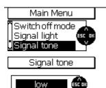
The signal tone is to confirm acquisition of readings and to confirm key action.
