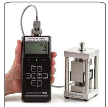
Handheld smart sensor indicator and high precision load cell
