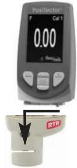
When powered-up, the **PosiTector** automatically determines which probe is attached and does a self-check.
