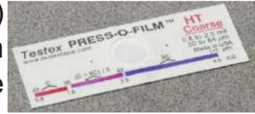
Placing the compressed tape (replica) into the **PosiTector RTR** gives a measure of the average maximum peak-to-valley height of the surface roughness profile. The Gage automatically subtracts the thickness of the polyester substrate from all measurements.
