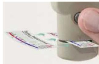
To position the tape, move the tape to the back of the probe and align the two dots (printed on replica tape) with arrows on both sides of the measurement opening.
