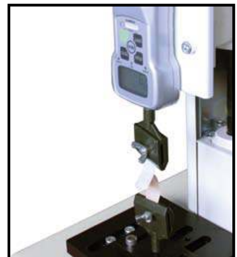
Stand with Optional Grip Performing Peel Test
