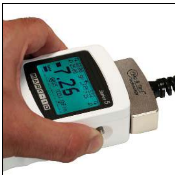
Fig. 3.2 Press both buttons on either side of the indicator housing to release the Plug & Test™ connector.
