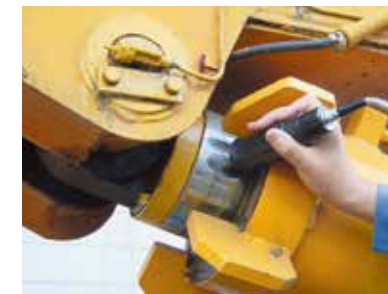
Diagnosing wear and tear using hardness measurements
