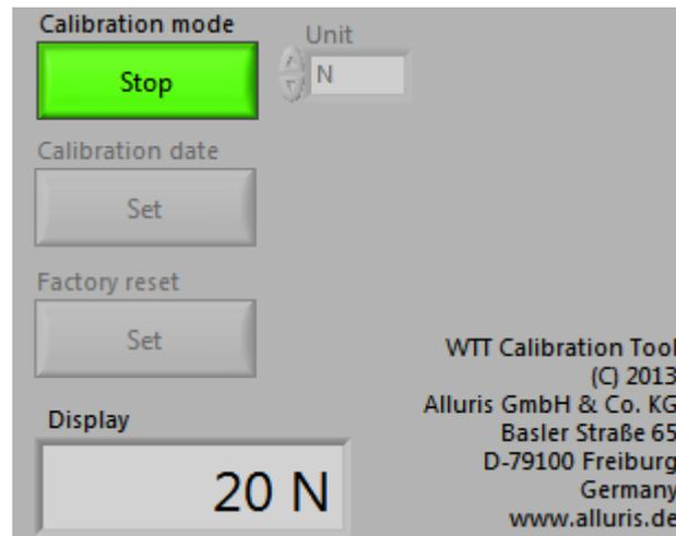
By starting the calibration mode the unit chosen in “Unit” field will be programmed to the device and it will be brought into the standard measure mode so there will be no annoying effects of the normal peak mode.
