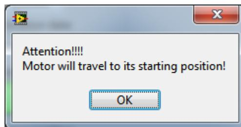
After acknowledge this message the motor starts to travel for 25 seconds (it's enough with the default speed of 100 mm/s) and will then be disabled until you turn off and on the pull tester.
