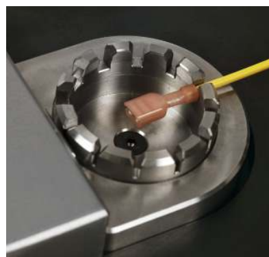
Rotating terminal fixture has 12 slots of different widths to accommodate various test materials. Slot widths range from 0.020" (0.5mm) up to 0.235" (6.0mm).
