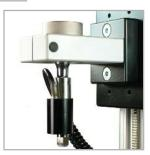
^ Optional AC1016 mounting kit mounts an MR54-200 or MR54-400 sensor to a torque test stand.
