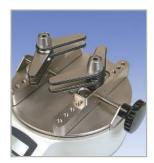
^ Optional CT003 adjustable jaws include 4 rubber-edged gripping arms per jaw. Arms may be independently repositioned in 45° increments to accommodate unique samples.
