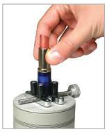
^ Low capacity Series R53 torque sensor is shown in a cosmetic packaging test.
