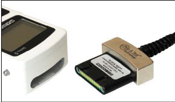
Fig. 3.1 Appropriate orientation of Plug & Test™ connector.
