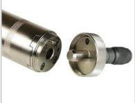
^ Series R51 feature unique interchangeability with three chuck attachment sizes as well as a bit holder. The attachment is mated to the main sensor body with a pin, while a threaded ring holds the attachment in place.
