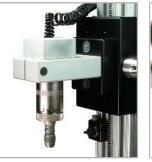
^ A Series R51 torque sensor is shown mounted to a model TSTM motorized torque test stand using optional AC1015 mounting kit.
