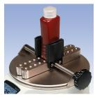
CT001 Flat jaws Set of rubber jaws for gripping
