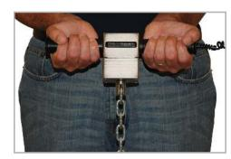
^ A Series R05 sensor is shown in a typical pull testing application. Chain is not included.
