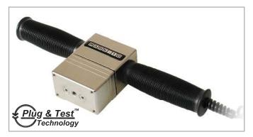
Series R05 fully enclosed smart sensors are designed for pull / push measurements. Useful in ergonomics testing, workplace safety testing, and general lifting or tension / compression requirements. Threaded holes are supplied to accommodate various mounting configurations and attachments. For up to 500 lbF [2,500 N]. Compatible with Mark-10 model 5i and 3i indicators (sold separately) through unique Plug & Test™ technology.
