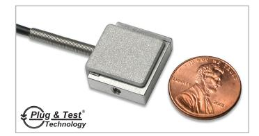
Series R04 smart sensors are designed for tension and compression measurement applications with tight space constraints. These extremely compact force sensors feature threaded holes on two sides, which can accept a variety of hooks and implements. Capacities available from 0.25 to 100 lbF [1 to 500 N]. Compatible with Mark-10 indicators (sold separately) through unique Plug & Test<sup>®</sup> technology. Includes a certificate of calibration with data.
