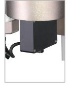
Series R03 sensor with shortened cable is shown mounted to an ESM1500LC test stand.\*
