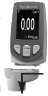
When powered-up, the **PosiTector** automatically determines which type of probe is attached and does a self-check.
