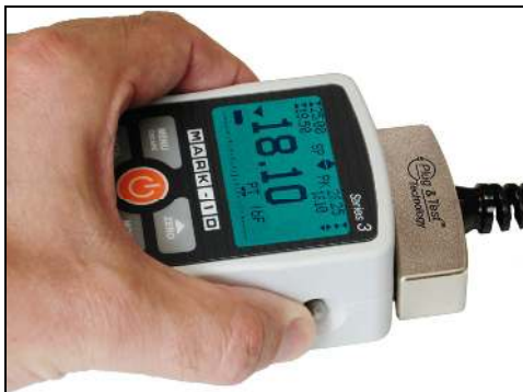
Fig. 3.2 Press both buttons on either side of the indicator housing to release the Plug & Test™ connector.
