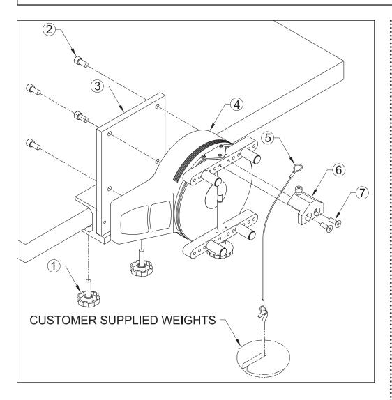
The AC1036 calibration kit is designed to permit the field calibration of any Series TT01 cap torque tester. The kit contains a complete set of attachments required to mount the tester to a bench, as well as the necessary brackets and cable to mount weights. Please note: weights are not available from Mark-10, and must be supplied by the user. The illustration at left depicts proper assembly. Please follow these instructions:
