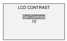
Press ENTER to modify the contrast. Select a value from 0 to 25, 25 producing the most contrast.
