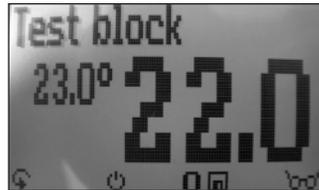
**NOTE:** If your gauge does not have a Test Block Curve, please select the Straw Curve. The readings should be as indicated below.
