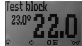
If the measuring value is blinking in grey, the value is beyond the stated specifications (*please read section 3.0 for possible reasons for errors*). If the measuring value is shown in black, the value is acceptable.
