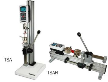
The TSA and TSAH are shown testing the peel force of a sample, with a Series 5 digital force gauge, and film & paper grips
