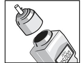
2. Select either the Cone Tip Adapter or the Funnel Tip Adapter and carefully place it on the shaft of the Screw-in Contact Adapter making sure to align the pin on the shaft with the slot on the adapter.
