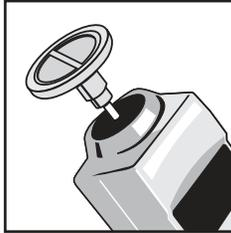
2. Rotate the *Operating Mode Selector Switch* to the desired unit of measure for surface speed or length.
