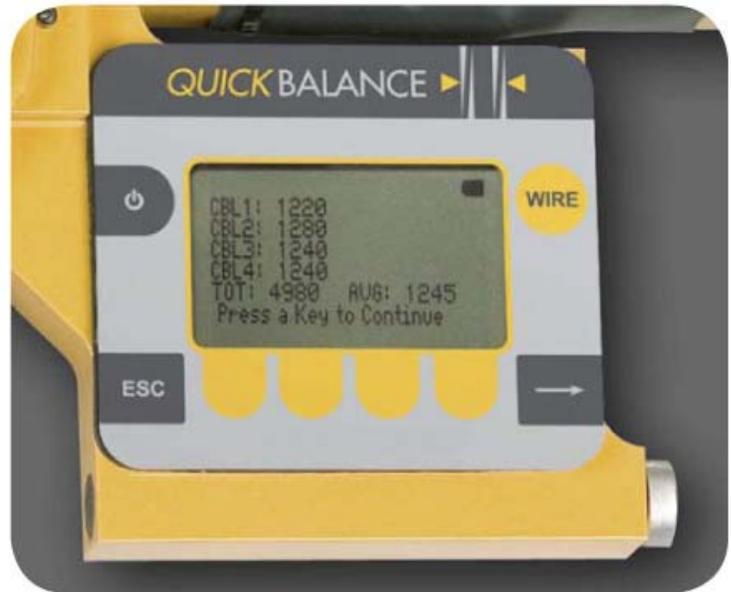
**Display showing cable tension summary screen.** To view a video demonstration of the QB-10000 click the button at right. *Note: you must have an active internet connection to view this video.*
