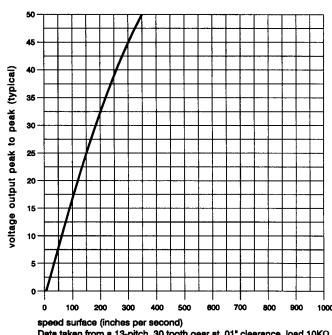
Data taken from a 13-pitch, 30 tooth gear at .01" clearance. load  $10 \text{K}\Omega$
